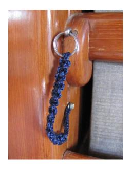
We use cotter pins to keep the fiddles from working their way loose when underway. This lanyard was used to keep the cotter pin from getting lost when the fiddle is out
